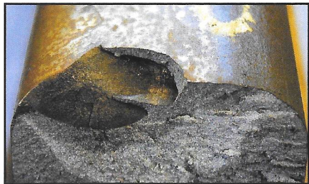
This Shows the Two Stage Development of a Crack from a Head Check.
