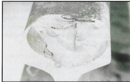
Surface & Fracture Face Appearance of Squat Type Defects
