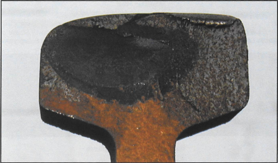
Broken Rail From a Head Check Defect (Originating from Gauge Corner)
