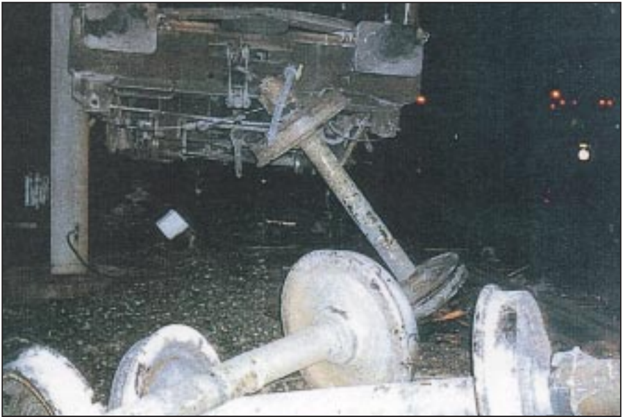
Photograph - The result of a cyclic top derailment.
