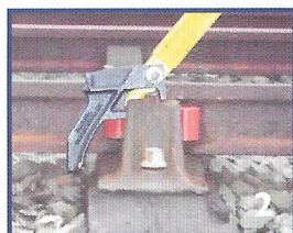
Panlock Insertion / Extraction Tool showing the four stages of insertion and extraction.
