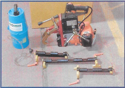
Cembre Rail Drill for drilling rails
