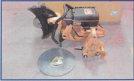
Rail Mounted Disc Saw for cutting rails
