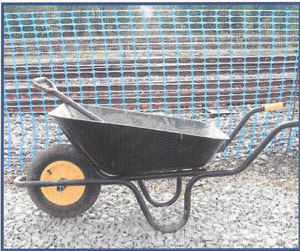
FIG 1.shows what looks like a typical wheelbarrow, however looking closely you will note the wheel is of the inflatable type. This allows us to move a load across the ballast freely. However it is not suitable for use on the 3rd rail system.
