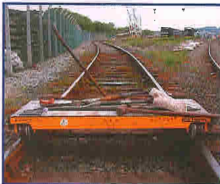
Fig 3. The device shown is known as a rail trolley, is more robust than the rail skate, running on both rails it allows the workers to carry larger items for example sleepers, timbers, large tools, small plant etc (only to be used with the permission of the signaller and under strict controls.)
