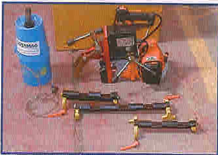
Cembre Rail Drill for drilling rails
