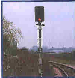
A three aspect signal capable of showing a red, yellow or green light
