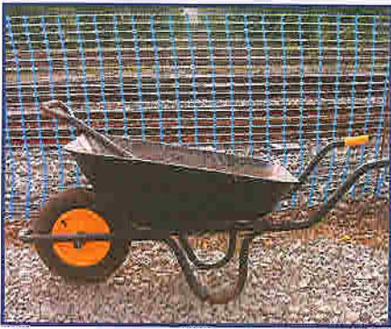
FIG 1. shows what looks like a typical wheelbarrow, however looking closely you will note the wheel is of the inflatable type. This allows us to move a load across the ballast freely. However it is not suitable for use on the 3rd rail system.
