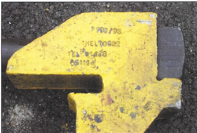
Fig 6 stamp marks on a Flatbottom TRJ clamp.
