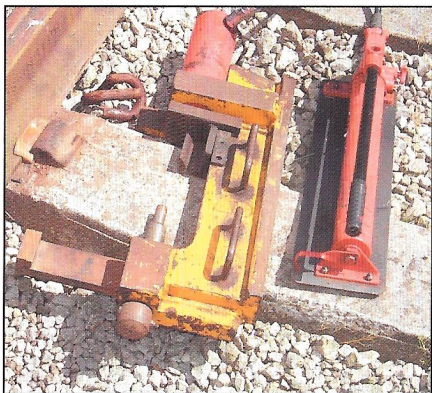
The Pandrol Rusty Clip Extractor for removal of frozen clips from concrete sleepers
