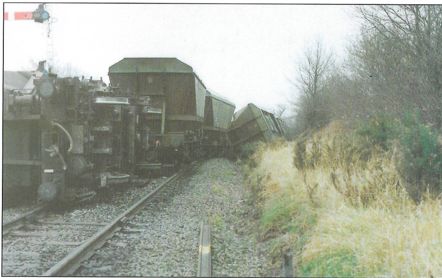
Fig.1. A gauge spread derailment
